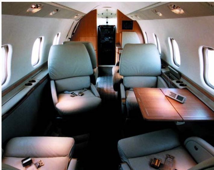
NEARLY SIX FEET WIDE, THE LEARJET 60'S STANDARD CABIN FEATURES FIVE EXECUTIVE SEATS, A TWO-PLACE SIDE-FACING DIVAN, A SMALL FORWARD GALLEY AND CLOSET AND A REAR LAVATORY.
