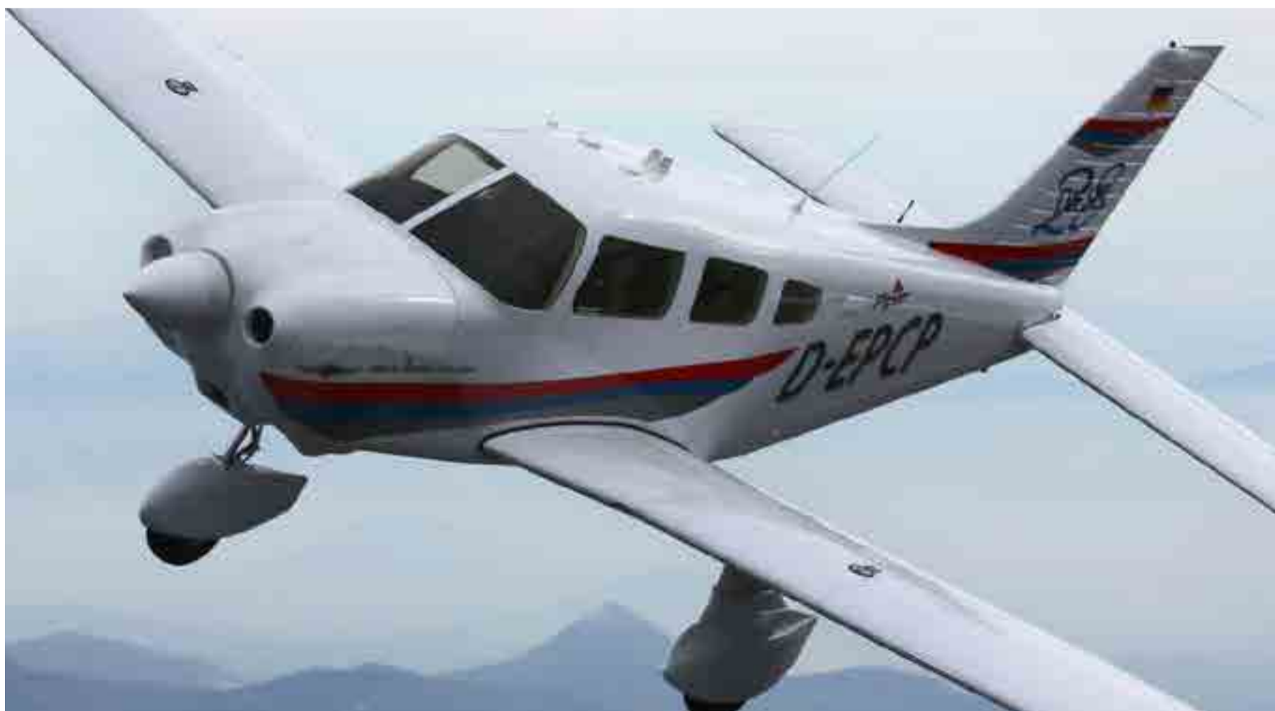
The Piper Archer DX, above, replaces the avgas Lycoming with a 155-hp Continental Motors CD-155 turbodiesel.
