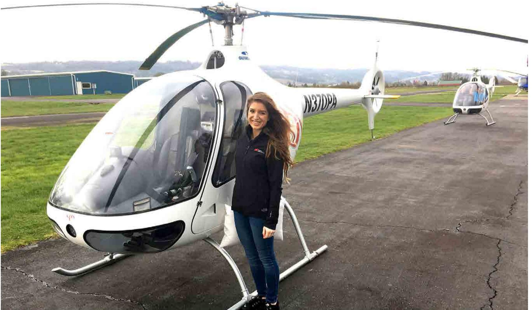
The Cabri's fenestron is one characteristic that will be an adjustment for pilots used to more typical trainers, such as the Robinson R22, according to AIN's Alexa Rexroth.
