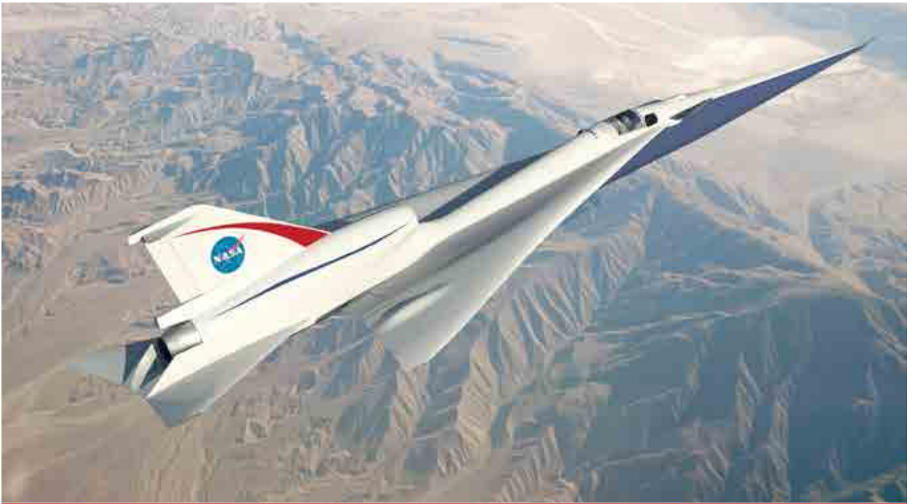
NASA and Lockheed Martin are teamed on the design of the Quest, slated to fly in 2021. It will test theories about how the design of the airframe can shape and muffle the sonic boom as it is perceived on the ground.
