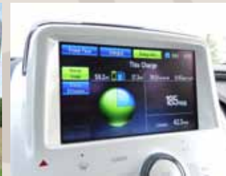
THE VOLT'S ENERGY MONITOR GIVES THE DRIVER A DETAILED PICTURE OF WHAT IS PROPELLING THE CAR AND THE RELATIVE CONTRIBUTIONS OF ELECTRICITY AND GASOLINE TO OVERALL EFFICIENCY.
