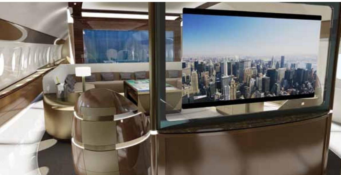
M&R Associates Design of Geneva has been in the private jet interiors business for a decade: more recently under its current brand name. One of its latest designs was this rendering for an Airbus A350 XWB. The cabin includes such coming technology as OLED video screens set into transparent walls and a large dining table with a thick marble surface through which "E-foil" light can pass, resulting in the interplay of diffused light with the crystal tableware.
